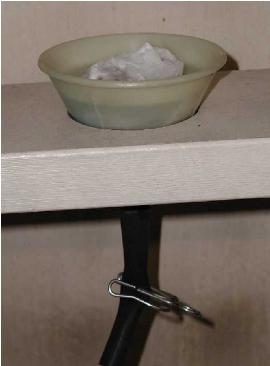
Figure 36. A Baermann funnel is a simple tool for extracting nematodes from material.
